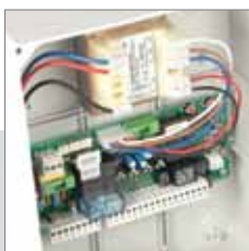
Electronic control unit with 433,92 MHz radio receiver
